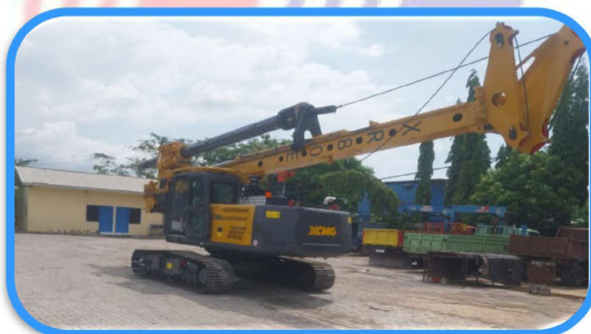
Drilling Machine (Borepile) XCMG/XR80E
